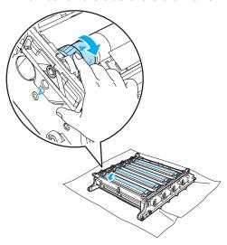
Hold the handle of the toner cartridge and slide the toner cartridge into the drum unit. Make sure that you match the toner cartridge color to the same color label on the drum unit, and make sure that you fold down the toner cartridge handle (A) once the toner cartridge is in place. Repeat this for all the toner cartridges.
